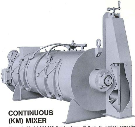
Shown is Model KM-600 (total volume, 21.2 cu. ft., typical capacity 18,000 lb. per hr.) Charging is through filler-opening at top end of mixer... working level is normally 50% of total capacity. Discharge is through slide valve at opposite lower end (see cut). Easy cleaning is accomplished through the two wide access doors at front side.
